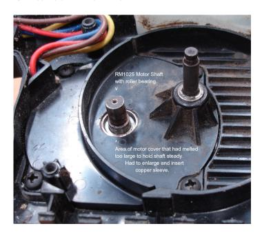
Locate a piece of  $\frac{1}{2}$ " rigid copper pipe, but do not cut off a piece yet. It will be easier to work with the larger piece of pipe first. Square off and remove any burrs from one end of your pipe. Sand inside and out until it fits over the bearing on the end of the motor shaft. It should be snug, but do not use pressure to press it on. This bearing is fragile and can be easily damaged from too much force.
