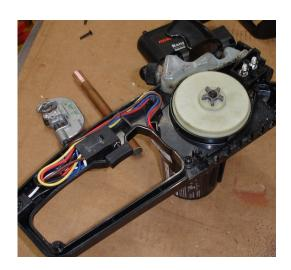
6. Lift off the white sprocket wheel from its axle.
