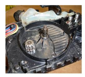
7. The large drive gear is positioned on the motor shaft. It should be held tightly in position by the plastic bracket or plate as shown in the above picture. It is held in position by four screws at the four corners. Lift off this large gear for a better look at the bracket.
