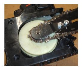
Remove the two nuts and the 'C' ring that attaches the bracket over the white sprocket disk. Remove the bracket and set aside.
