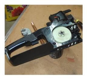
Remove three screws holding the handle cover to the saw assembly.
