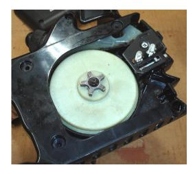
4. Remove the chain tightening assembly that surrounds the two bar bolts. It is held by one Philips flathead screw.
