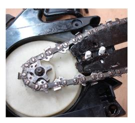
3. Remove the saw chain and bar.
